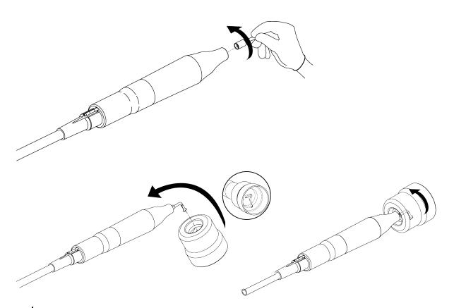
The wrench is a sliding torque wrench. After a few turns, the wrench will seem to slide or turn without resistance. This means the tightening torque is reached.
